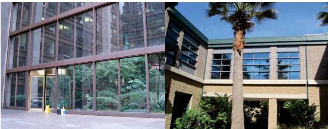
Indoor vegetation (left) and reflections of vegetation in a private courtyard (right) situated in close proximity to untreated glass façades are likely to attract birds and increase the chance of collisions. Image credits: Christine Sheppard
