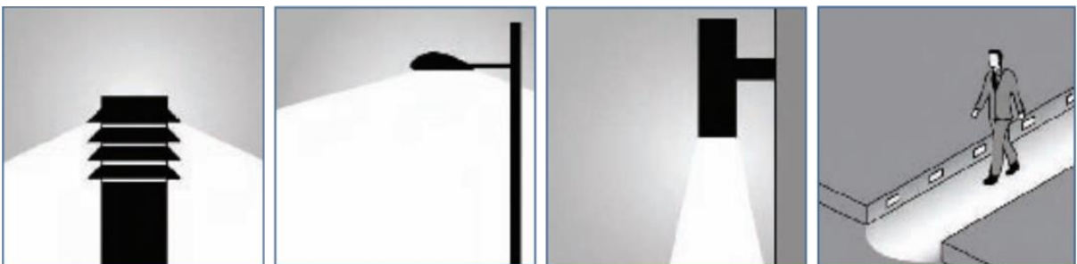
Examples of various external lighting fixture designs that minimise spill light. Image credit: San Francisco Planning Department 2011
