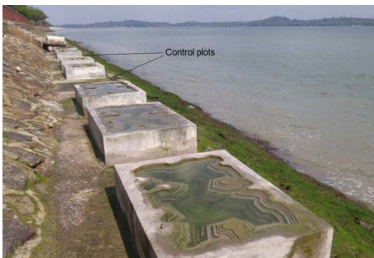
Fig. 3. The tidal pool units positioned in a randomised layout with control plots (empty slot without any tidal pool unit).
