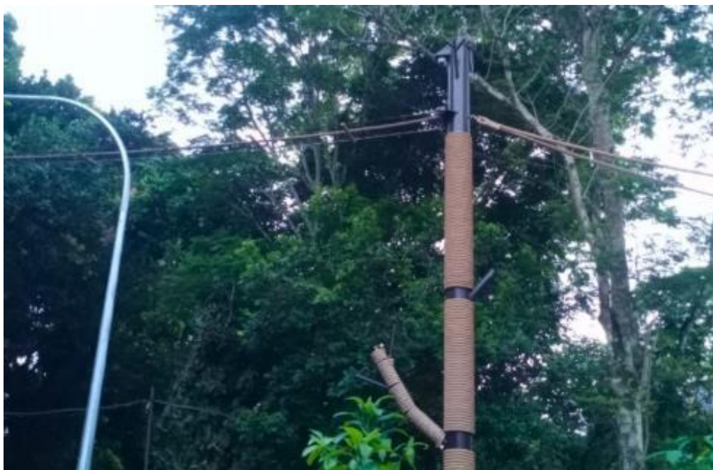
Fig. 6. Animal monitoring camera installed on Arboreal Crossing for long term biodiversity monitoring.
