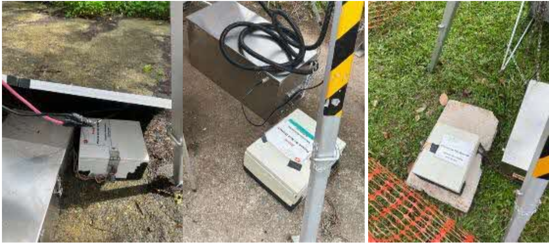
Figure 11-2. Pictures of the on-site baseline ground-borne vibration monitoring equipment
