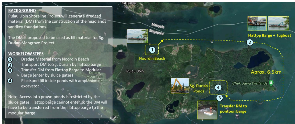
Figure 3-17 Overview of transportation process of the dredged material to the Project Site
