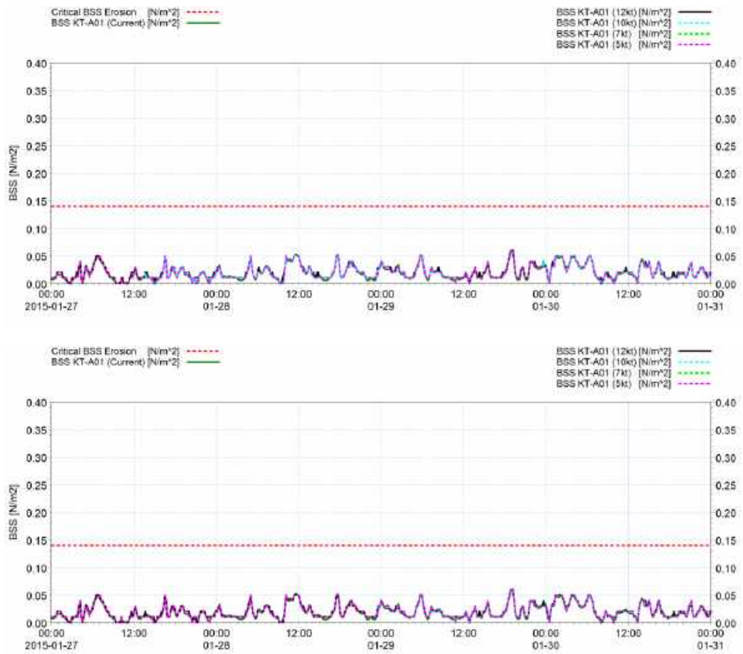
Figure C.13 Time series of BSS generated by current (HD) and ship wake at Area 1 Pulau Ketam shoreline (KT-A01). Each line represents BSS at different vessel speed (12 knots, 10 knots, 7 knots, 5 knots): vessel inbound (top) and vessel outbound (bottom). Potential erosion occurs when BSS > 0.14 \text{ N/m}^2
