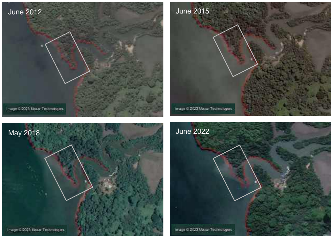
Figure 5.11. Area of focus D, southeast of the proposed jetty site. Signs of erosion can be seen from June 2012 to June 2022 within the grey box
