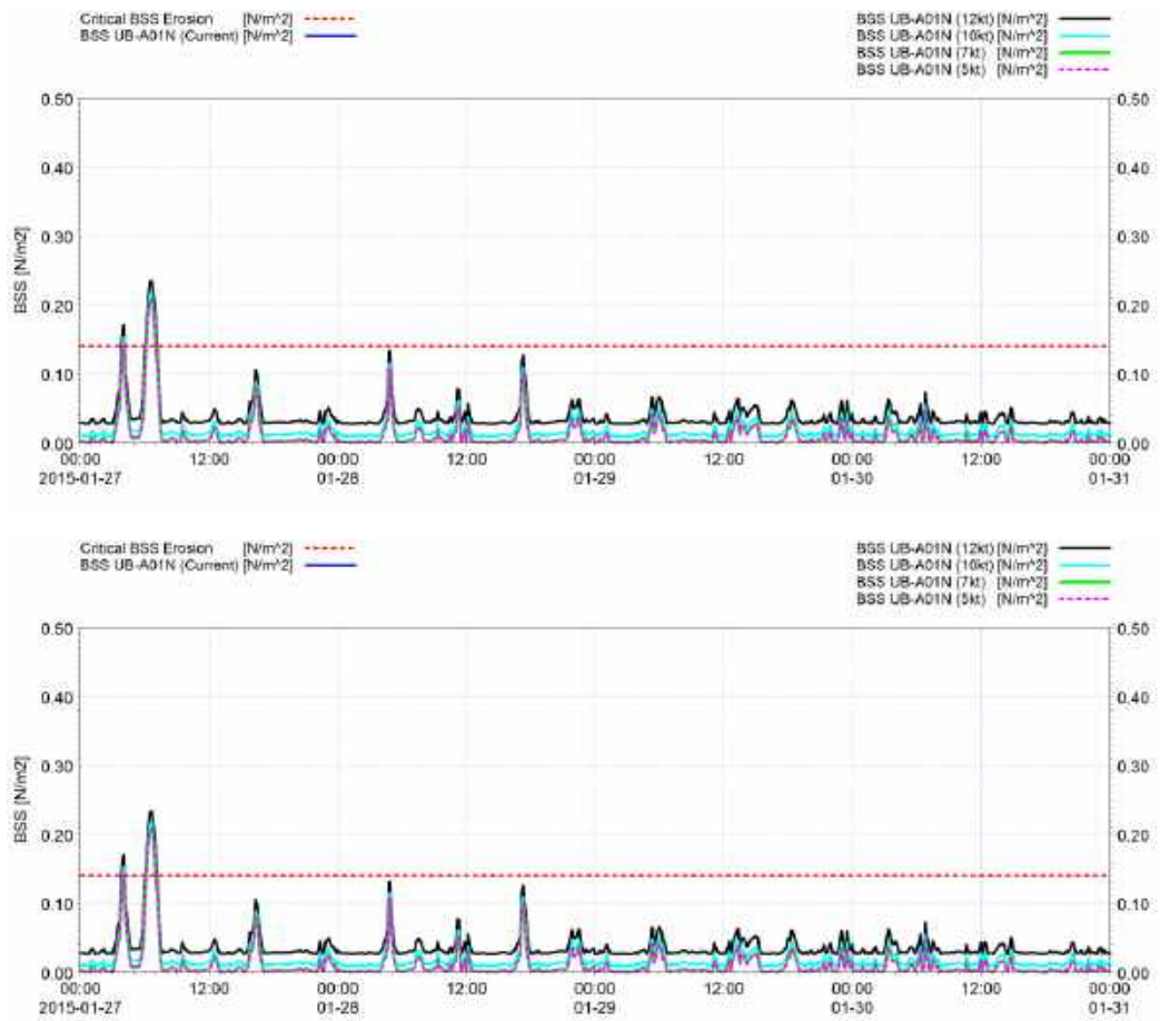
Figure C.8 Time series of BSS generated by current (HD) and ship wake at Area 1 intertidal zone for Pulau Ubin shoreline (UB-A01N). Each line represents the calculated BSS cause by vessels travelling at varying speeds (12 knots, 10 knots, 7 knots, 5 knots): vessel inbound (top) and vessel outbound (bottom). Potential erosion occurs when BSS > 0.14 \text{ N/m}^2
