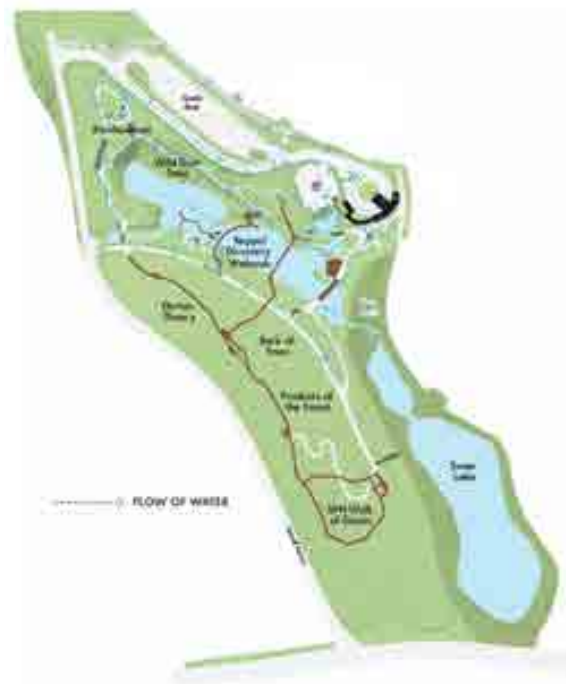
Fig. 4. Rainwater falling onto the catchment area of the Wetlands is channelled through a series of bioswales and siltation ponds, eventually finding its way through the Dell and into Swan Lake.
