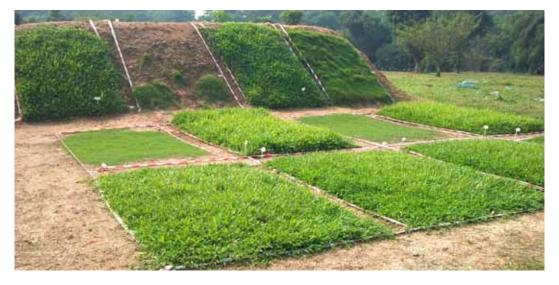
**Fig. 4** Experimental plots after 10 weeks of hydrosprigging application
