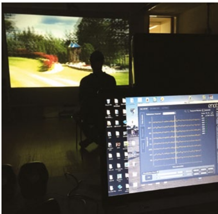
6. EEG data acquisition with a wireless mobile device.
