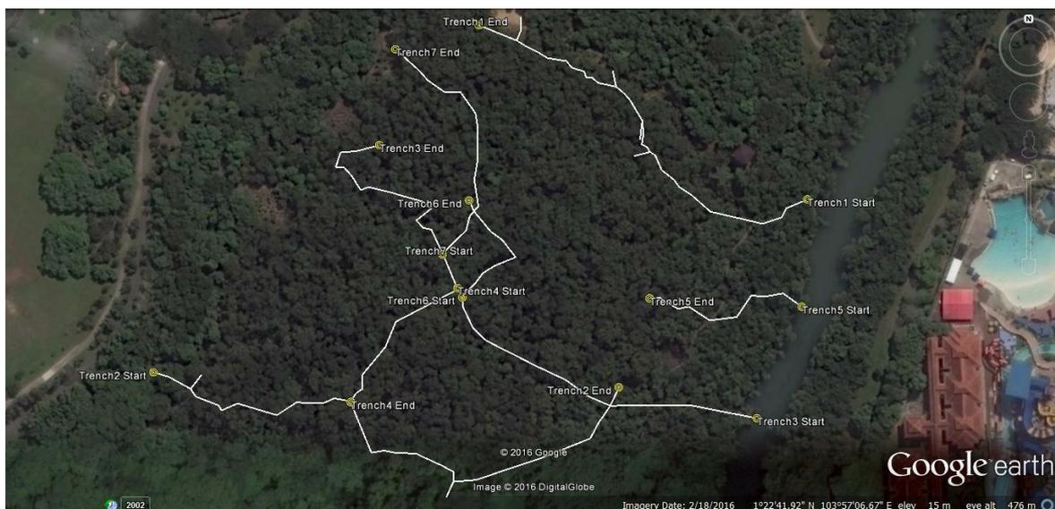
Fig. 4. Map of trench lines using GPS. (Image credit: Google Earth)
