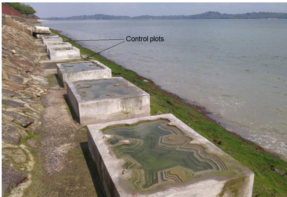
Fig. 3. The tidal pool units positioned in a randomised layout with control plots (empty slot without any tidal pool unit).
