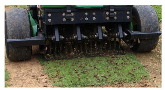
Fig. 1 Hollow-tine aerification
