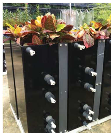
Figure 7 Photo on the top left shows the experimental setups under a transparent pitched roof structure at Pasir Panjang Nursery in 2010. Photo on the top right shows the typical bioretention columns with trial plant species growing in them. Schematic diagram of bioretention columns indicating dimension details and substrate layer configurations.
